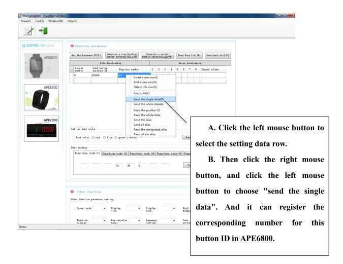
3) Send the whole data (APE6800 needs to be set in "download" mode) In any area of the form, click the right mouse button to select "send the whole data"—pop up the dialog "command execution success"—click "OK" to exit. The all information of the buttons uploaded is registered successfully in the watch.
